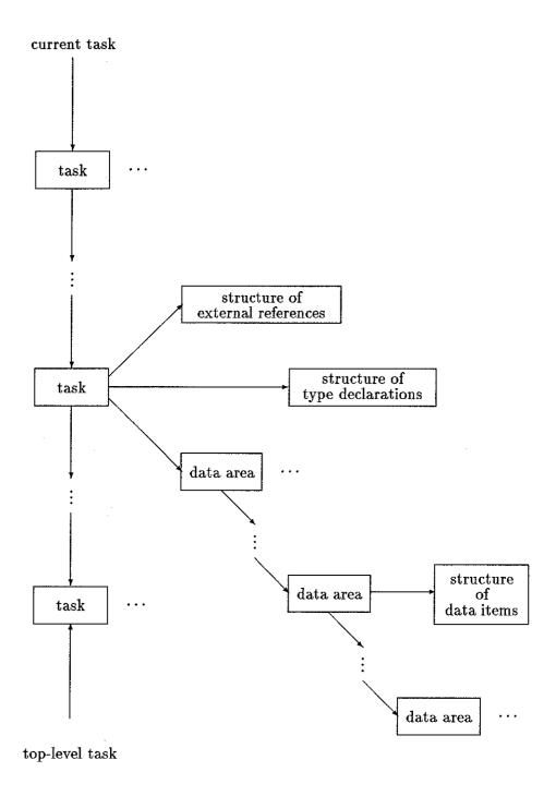
Figure 1: Internal representation of an EPP program.
